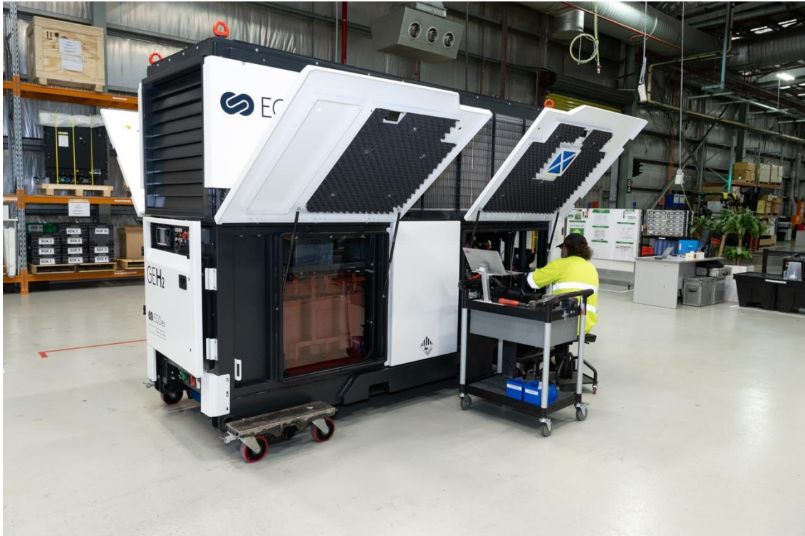
File: 24 Toyota Hydrogen Generator Event 26th Feb DSC_0641 Caption: A Toyota worker assembling the EODev GEH2 generator at Toyota' Altona production facility
