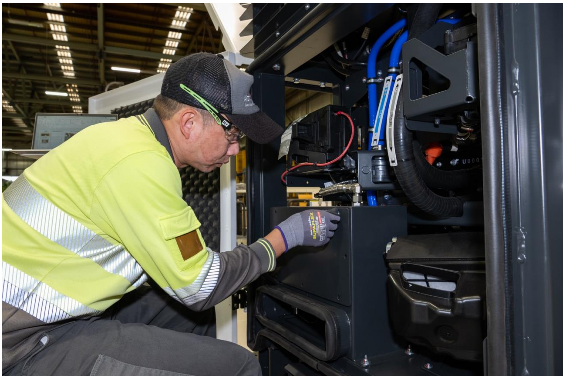
File: 24 Toyota Hydrogen Generator Event 26th Feb DSC_0660 Caption: A Toyota worker assembling the EODev GEH2 generator at Toyota' Altona production facility
